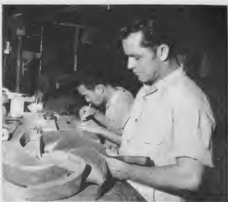
PATTERNS, such as that of the pump impeller on which Joseph Maduro is working at right, are the heart of any foundry project. Mr. Maduro and E. Paula (left), frequently work to thousands of an inch in the patterns and cores they make.
